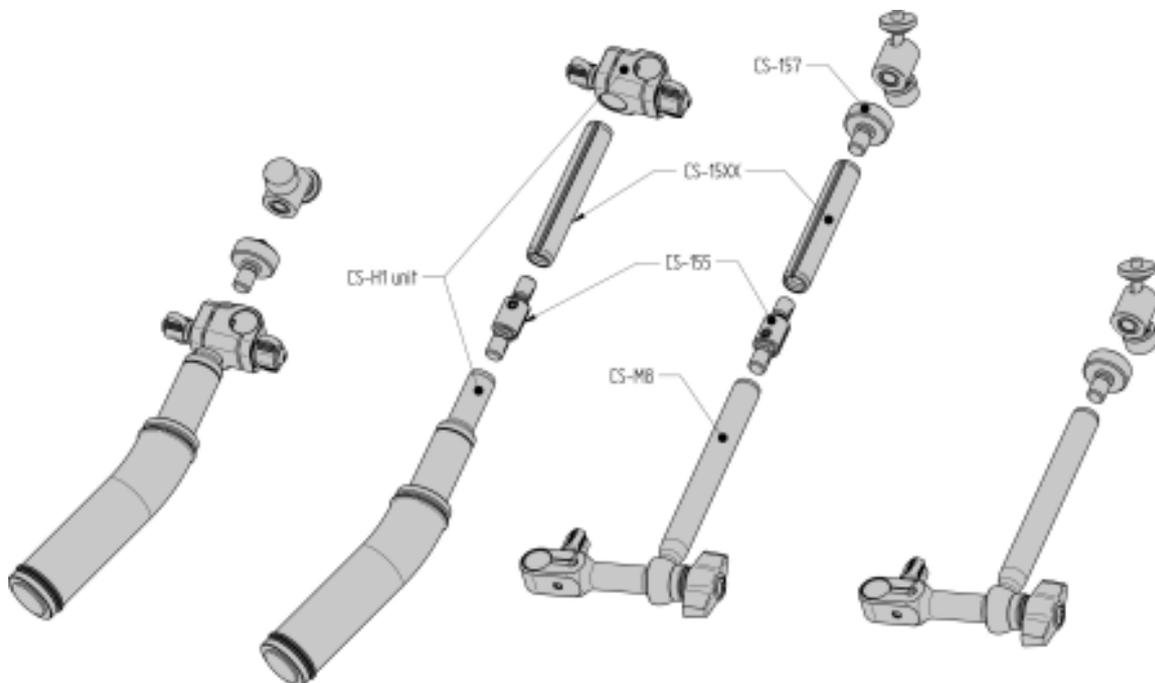
The CS-M8 is a separate monitor/microphone/light stand which couples to the 15mm iris rod. The CS-H1 handle can be extended using a CS-155 connector and a CS-15XX iris rod.
