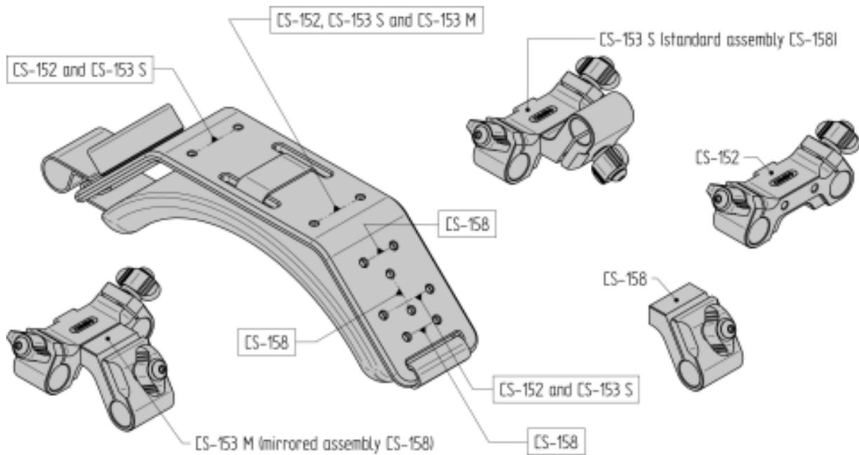
The image above shows the different mounting options of the CS-P1 shoulder pad. The CS-152/153 and the CS-158 can be mounted directly to the CS-P1 shoulder pad.
