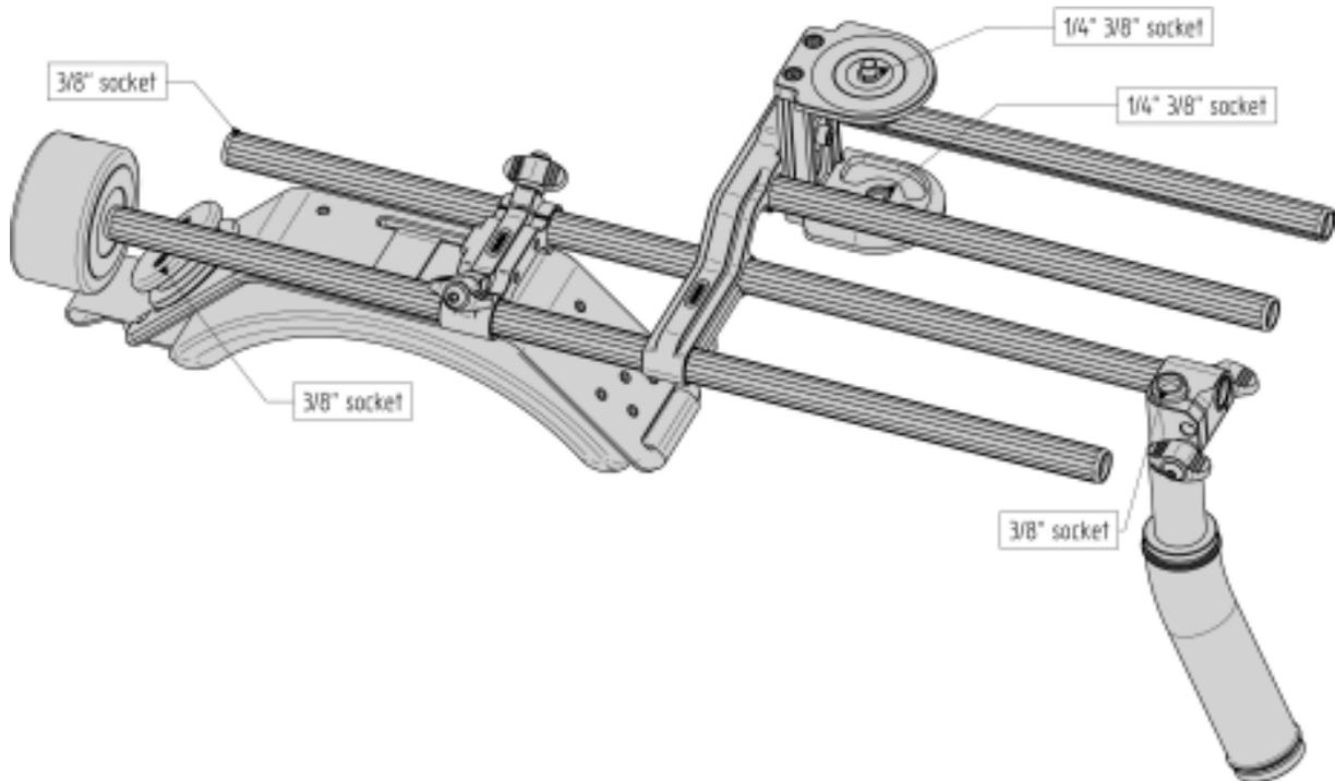
The CS-15XX iris rods feature 3/8" sockets which can be used for mounting attachments.
