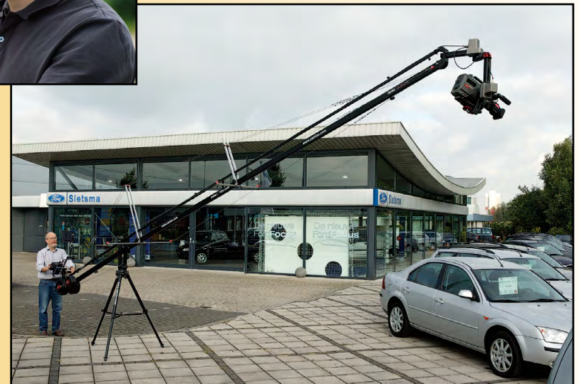
V40 in use on location with optional PT-900 and TVB-100 V-40 is extended with 4 meter, supported with cable stabilisation system VCSS-400-60, V-46 and LCD screen
