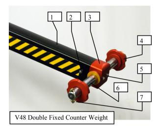
The End Cap of the V40 tail has to be removed first. The V48 weight block (3) fits the profile the same way, fixed with the locking screw and nut (2) nut through the existing holes in the Tail Beam (1).
