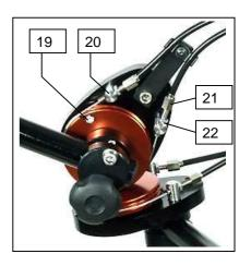
the cable attachment at the MPT Head have the longer stud at the same place. This determines the turning direction of the camera.
