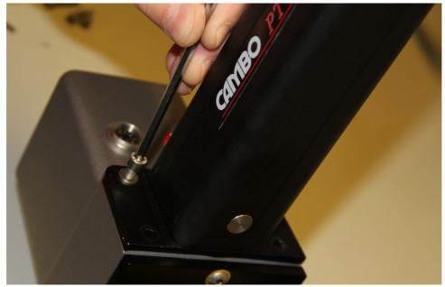
3. ASSEMBLE THE PLATES USING THE LONG HEX SCREWS (PROVIDED WITH THE PT-143 UNIT) WITH A 4MM HEX-KEY
