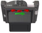
Now slide the lever to the right most position, this will lock the pins of the AFi mount.
