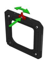
Make sure the lever is in the left most position, place the Afi(-II) digital body. When the pins are fully inserted, lock the mount by pressing the locking pin of the lever, now you can slide the lever to the right most position.
