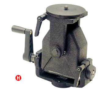
H Cambo 3-D Gearhead (SCH) Provides 140° of self-locking tilt, 90° forward and 50° back. 180° manual side-to-side tilt movement with adjustable resistance. (Includes 3/8" threaded mount.)
