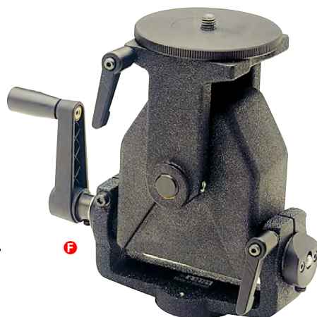
F CAMBO SCH 3-D GEARHEAD Cambo's SCH precision-gear movement has important advantages over standard friction-locking ballheads and other 3-D schemes. Minute adjustments are precise and controllable. And because movement is geared, it is self-locking. The Cambo 3-D Gearhead provides 140° of self-locking tilt, 90° forward and 50° back. 180° manual side-to-side tilt movement features adjustable resistance. Mounts to universal 3/8" threaded tripods.
